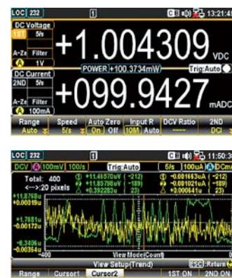
The dual measurement function has always been a unique feature of GW Instek digital multimeters, allowing two measurement functions to be performed simultaneously and displaying the test results separately so as to greatly improve the test speed of the multi-functional measurement tasks.
