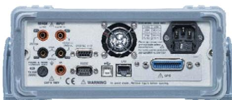
For system integration applications, the GDM-906X series is equipped with RS232, USB and LAN as standard communications interfaces, and GPIB is an option (can be installed by customer) to meet the requirements of different system integrations. Data transfer rate is up to 10k readings per second (GDM-9061) or 1k readings per second (GDM-9060) via USB/LAN/GPIB interfaces.
